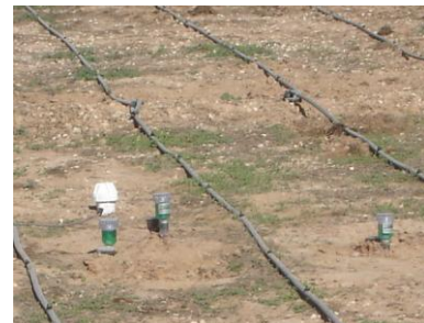
Fig.28: Measuring soil moisture with tensiometers
