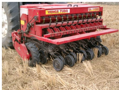
Fig. 23: Tractor-mounted direct seeder sowing wheat into rice residues in Egypt Source: FAO 2008
