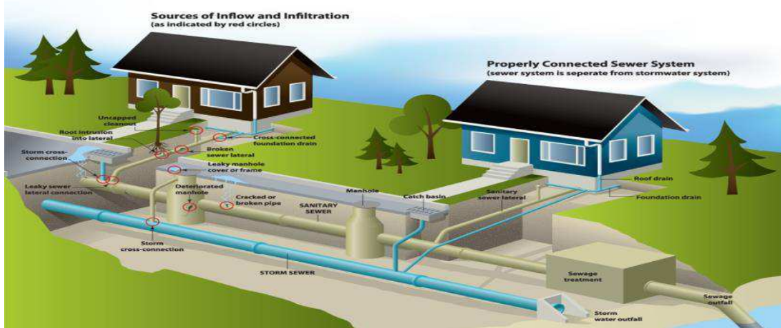
Figure 13: Separate sewer networks ( http://www.utilitieskingston.com/wastewater/Overflows.aspx )
