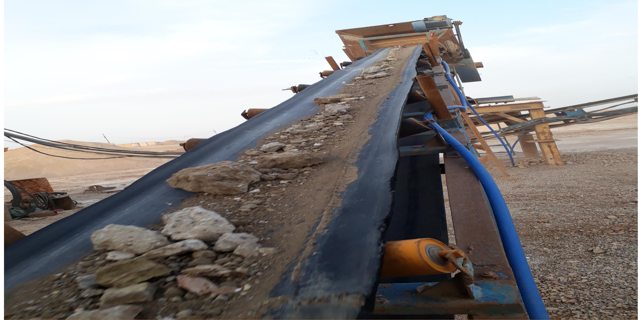
Photo 8. show the demolition waste subbase on the belt of crusher
