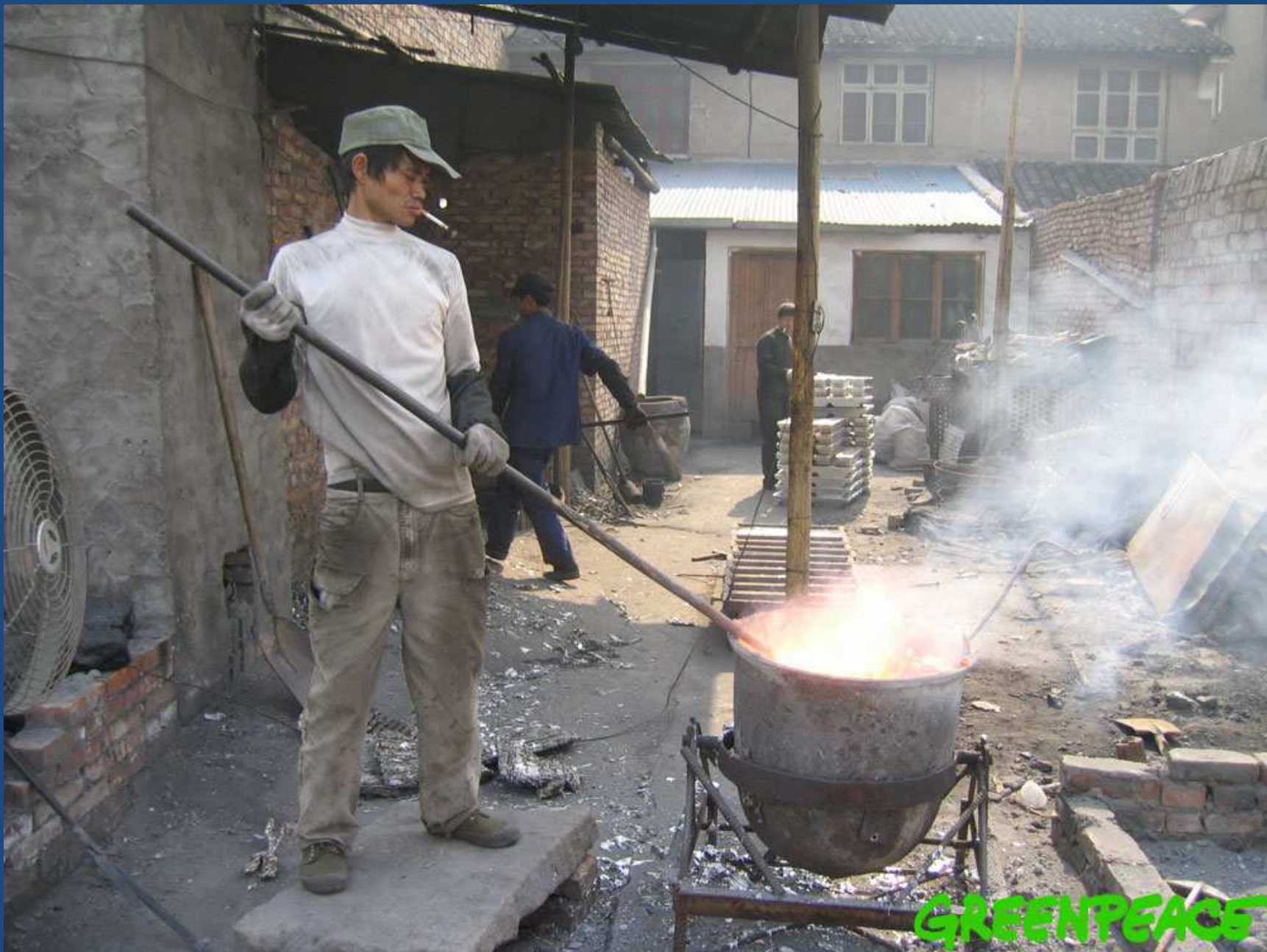
Chinese man smelts computer parts in the open air to extract metals. Open air burning of computer waste releases large amounts of toxic fumes.
