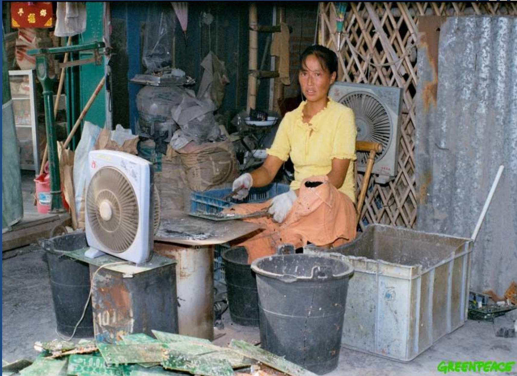
Chinese woman smelts computer circuit boards over an open stove to extract metals. The fan is vain attempt to disperse the highly toxic fumes created by the smelting.
