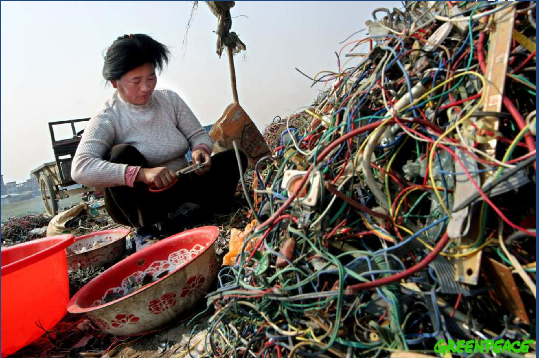
A migrant worker strips plastic from wires to extract useful metals. The plastic on the wires is often PVC which contains toxic chemicals and produces large amounts of pollution when disposed, often by burning in the open air.
