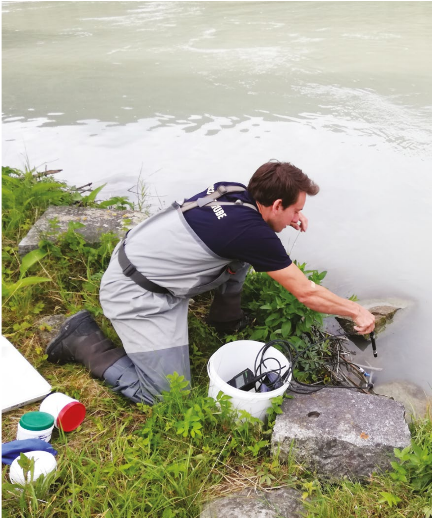
Joint Danube Survey 4, measuring physicochemical parameters
