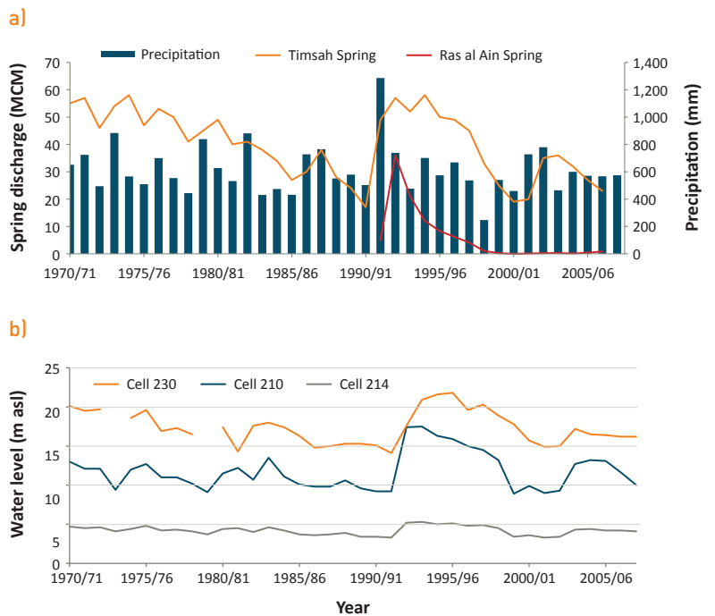
Figure 3. (a) Annual discharge of the Timsah and Ras al Ain Springs and average annual precipitation in the Western Aquifer Basin area (1970-2007); (b) annual water level fluctuations of different groundwater cells in the Israeli part of the basin (1970-2007)
