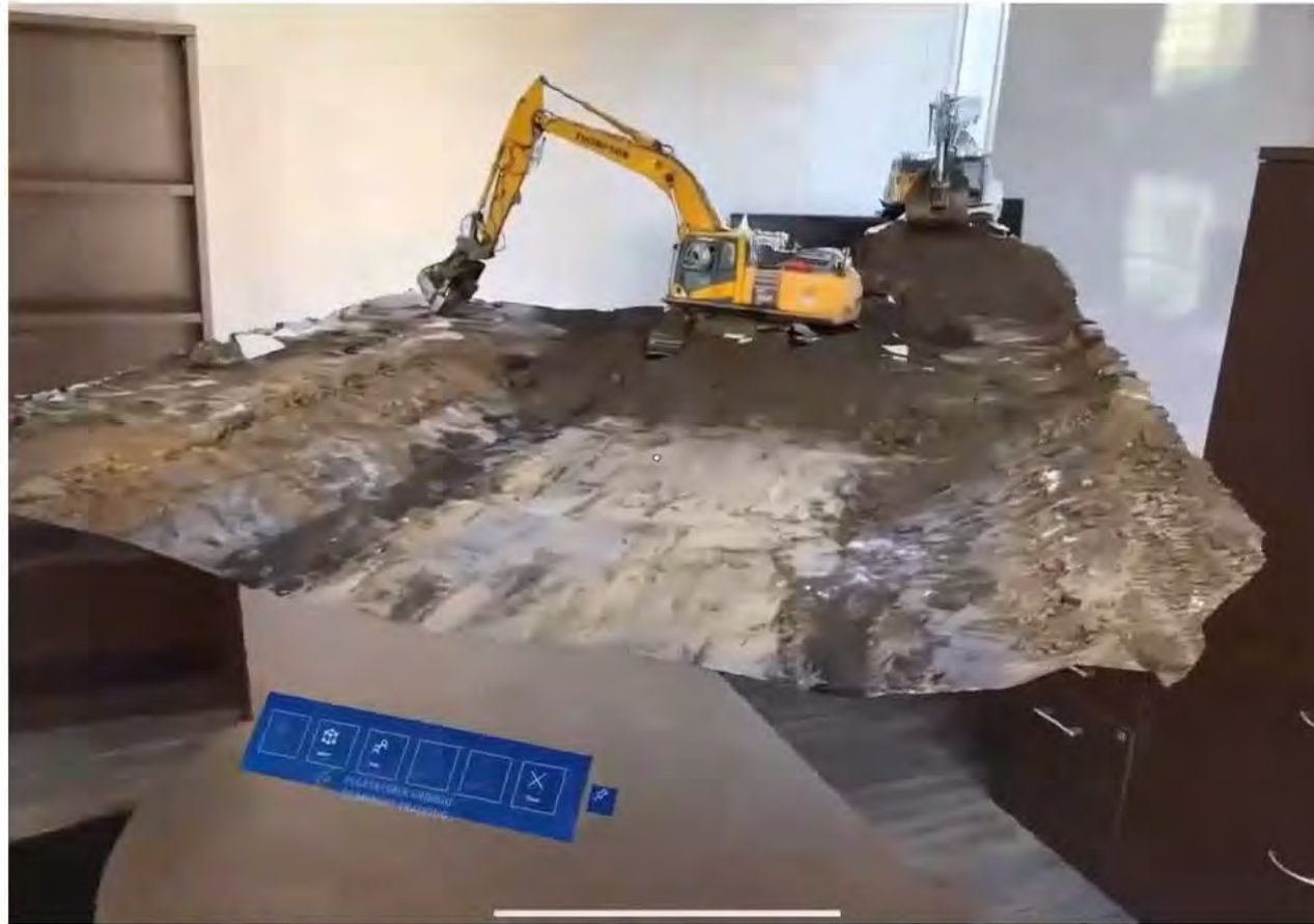
Photogrammetry model from Cell Phone photos
