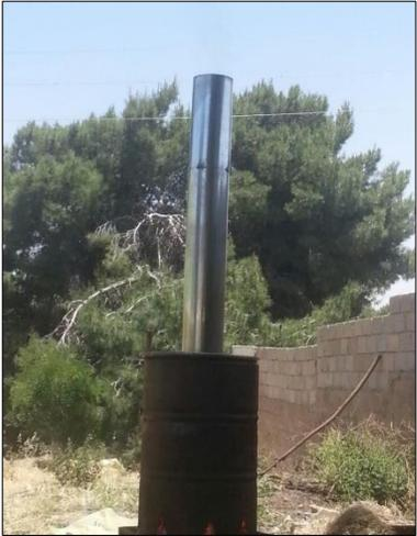
Figure 18. JBRI pyrolysis reactor
