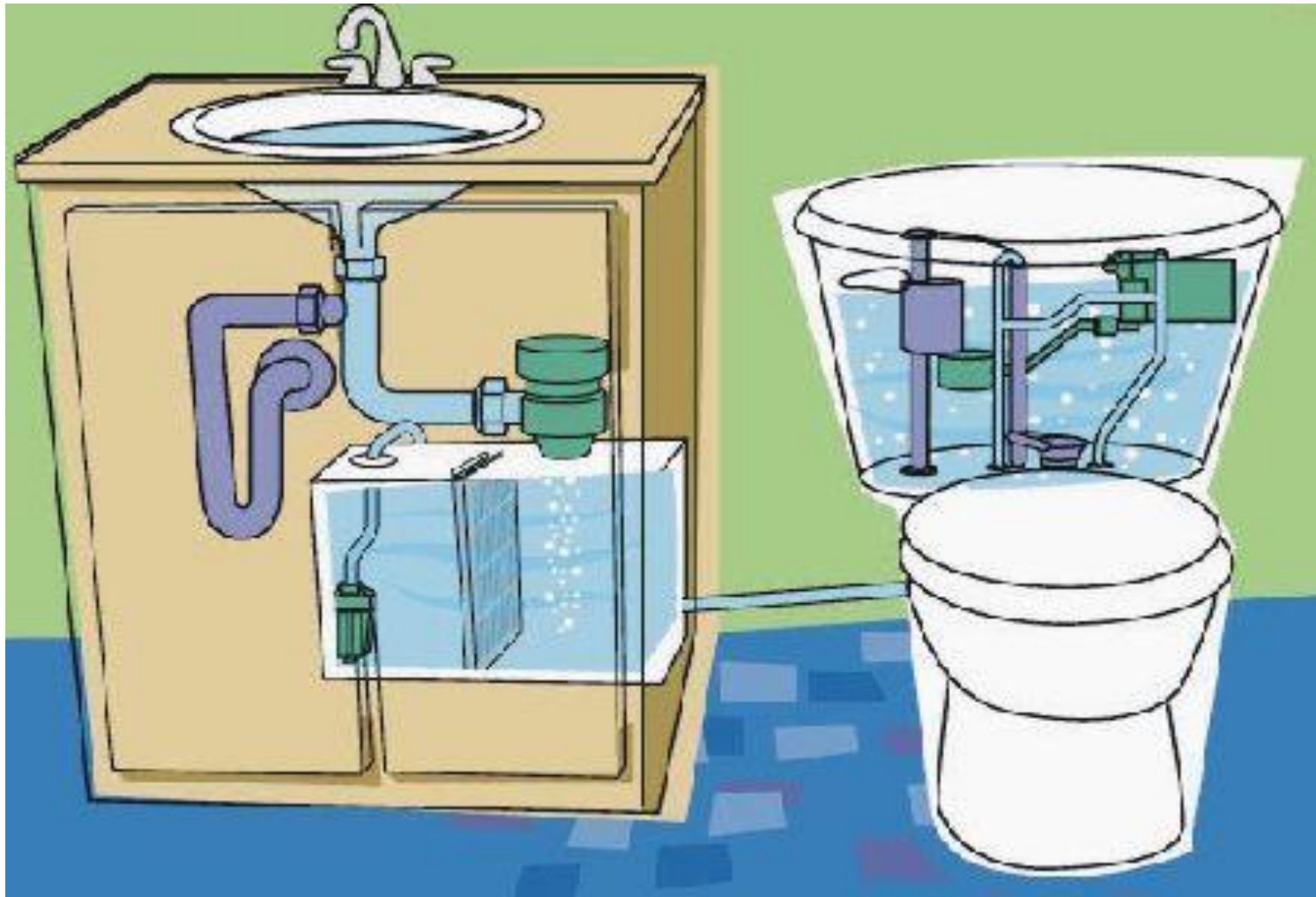
The Aqus(TM) WaterSaver technology which uses sink greywater for toilets; Source: Lepisto, 2006.
